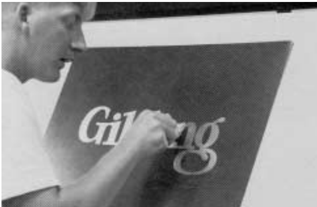
Figure 5. Engine-turning the gild
