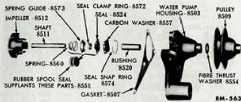
Fig. 46—Water Pump (Bushing Type), Disassembled
