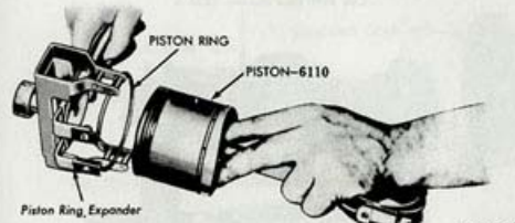
Fig. 27—Installing Piston Ring on Piston
