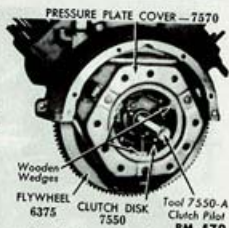
Fig. 61—Installing Clutch Disk and Pressure Plate
