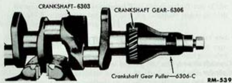
Fig. 12—Removing Crankshaft Gear
