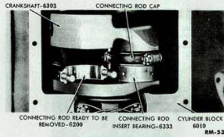
Fig. 7—Connecting Rod and Piston Ready to be Removed
