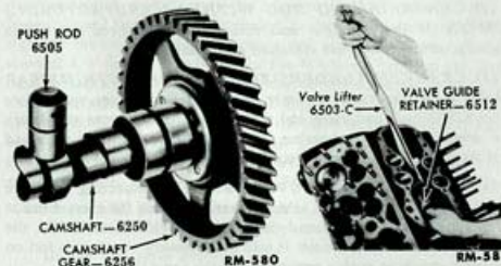
Fig. 63—Push Rod on Heel of Cam
