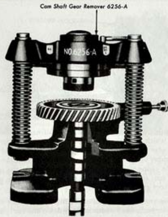
Fig. 28—Removing Camshaft Gear (Press-on Type)
