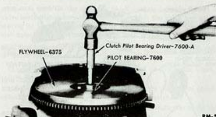
Fig. 14—Replacing Pilot Bearing
