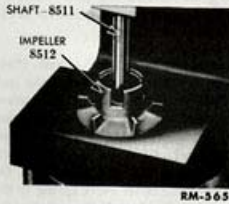
Fig. 47—Pressing Shaft Into Impeller (Bushing Type)
