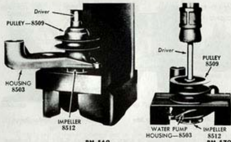
Fig. 51—Pressing Pulley on Water Pump Shaft (Bushing Type)
