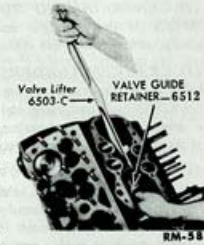
Fig. 64—Installing Valve Guide Bushing Retainer
