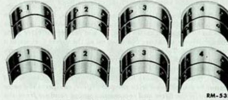
Fig. 8—Identification Marks on the Connecting Rod Bearings
