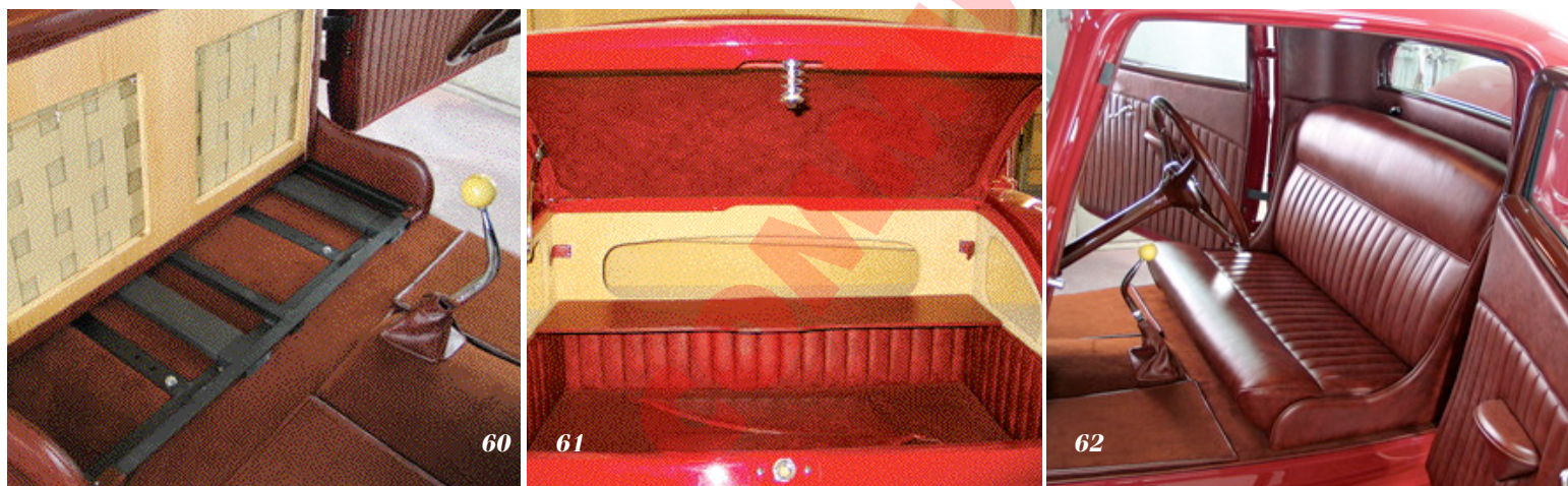
60 The interior is in the process of being completed. 61 The trunk panels are being assembled, and even the luggage compartment is perfectly finished on this car. 62 Here's the finished interior. All that's needed inside is a driver!
