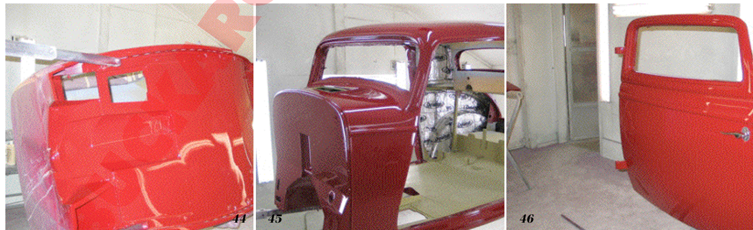
44 The underside of the body was the first in a long line of parts to be sprayed. 45 Here is a shot of the body after paint; Fastlane Red gives the car a whole new appearance. 46 Every part of this coupe was worked to perfection prior to receiving the final coats of paint.
