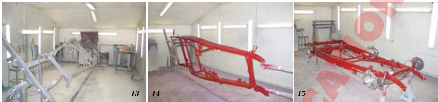
13 Once the chassis had been completely mocked up, it received a coat of primer. The next steps will be more sanding and the application of beautiful red paint. 14 This is the newly sprayed chassis in all its red glory. The detail work on the chassis is as nice as the topside. 15 The chassis has now been reassembled and awaits a set of rollers and a drivetrain.
