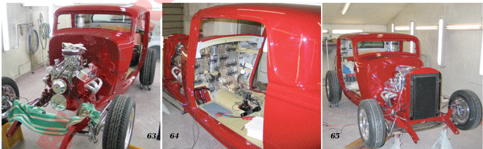
63 The color is Fastlane Red, and the body has been reunited with the chassis and drivetrain. 64 The insulation, pedals and shifter have found a home in the coupe. At this point, the wiring is a work in progress. 65 The radiator, shroud and electric fan are the next pieces to go into place.
