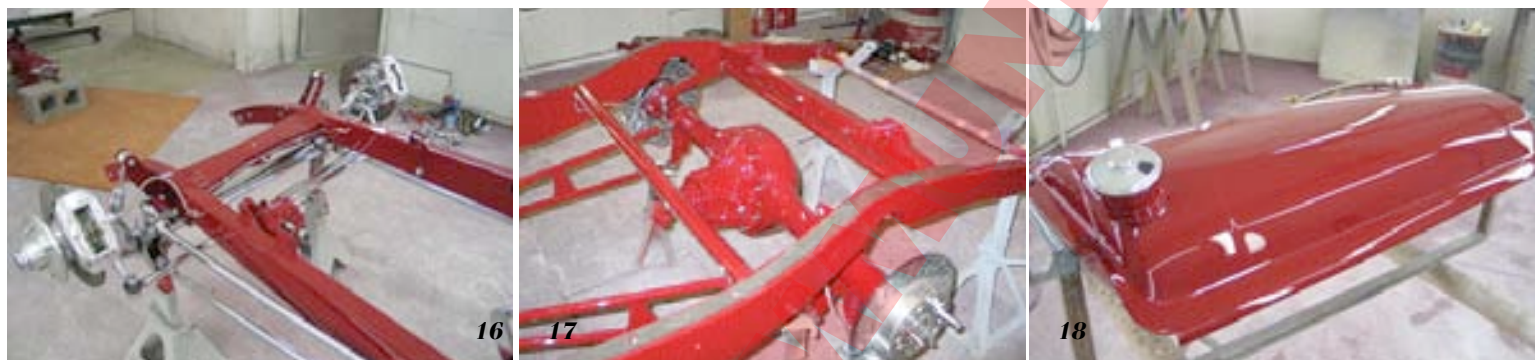
16 The new axle has been installed along with the brakes. Once again, attention to detail is everywhere. 17 The body welt has been laid down on the chassis, awaiting the body. 18 This has to be one of the slickest fuel tanks ever. The fuel neck has been custom-built to allow for a cleaner fuel-entry point.
