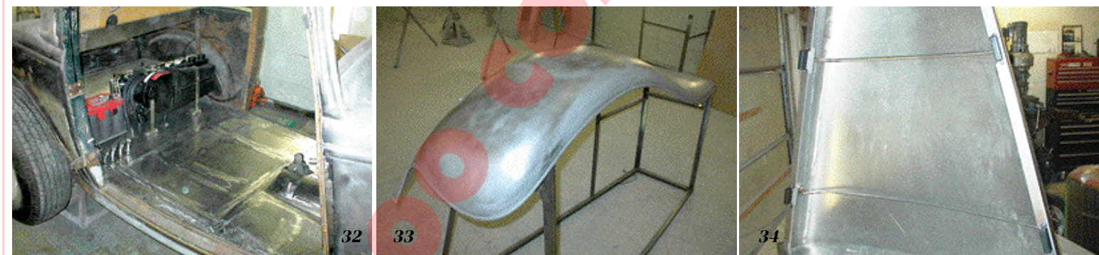
32 The old floorboards were cut out and replaced with new units, ensuring that there was no rust left in the car. 33 Every part on the coupe received hours of labor to finish it to perfection. 34 The fabricators at Fastlane built the custom three-piece hood for the '32.
